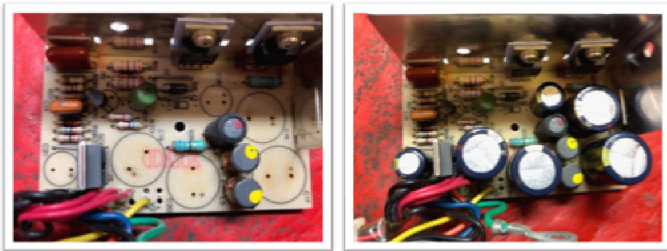
Figure 4 – Output Capacitors location
